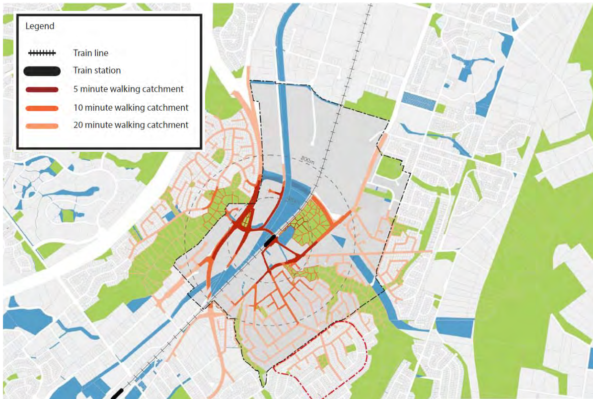
Figure 4-9 Leumeah Station walking catchments
