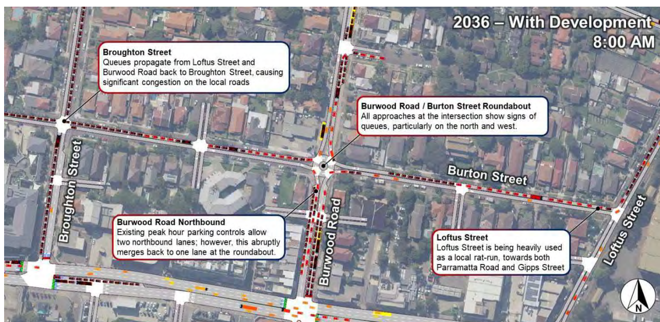
Figure 4-19: Burwood Road / Burton Street Roundabout Pinch Point
