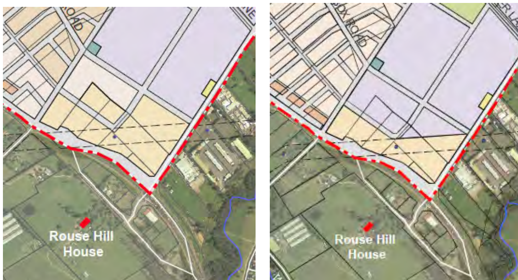
Figure 3-9 Corner of Windsor and Annangrove Roads, draft ILP and revised draft ILP – the area of light industrial is increased up to the ridgeline, reducing the area of large lot residential. The lot size is also reduced to 2000m 2 .
