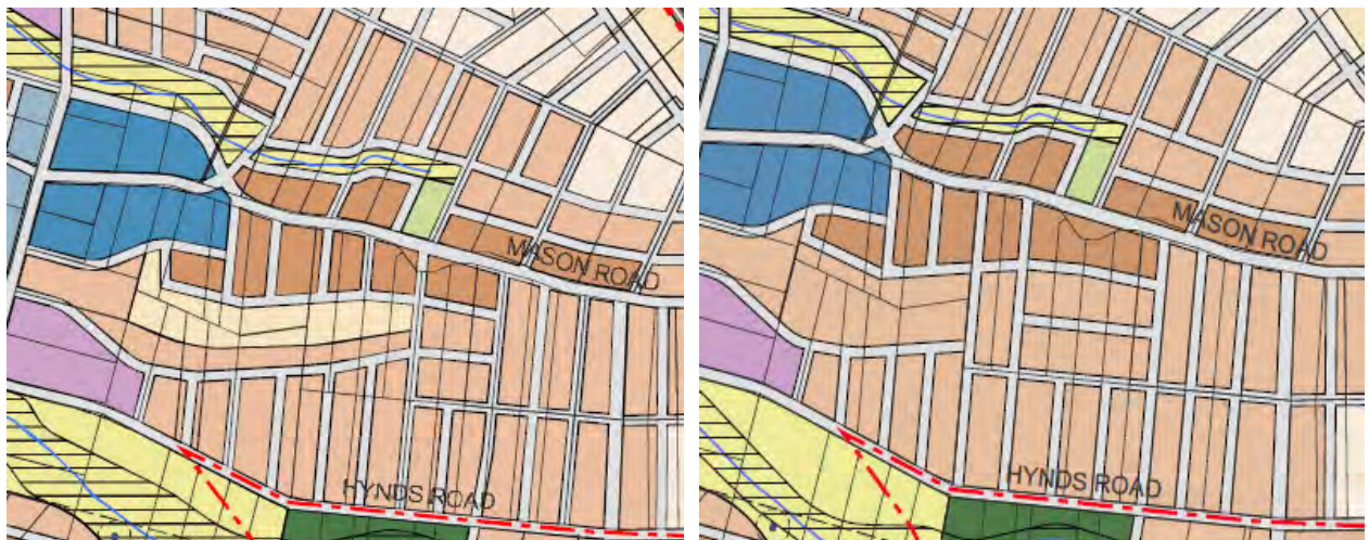
Figure 5-3 Second exhibited draft ILP and final ILP – large lots on ridgeline (cream) replaced by R3 Medium Density (mid brown).
