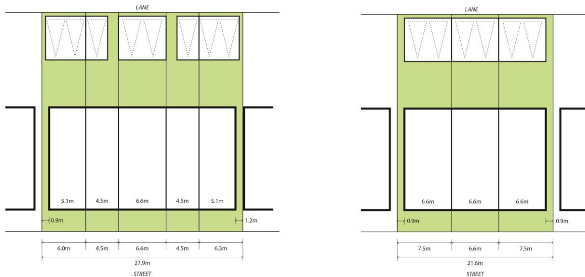
Figure 3-4: Two examples of lot subdivision for 'sets' of attached or abutting terraces.
