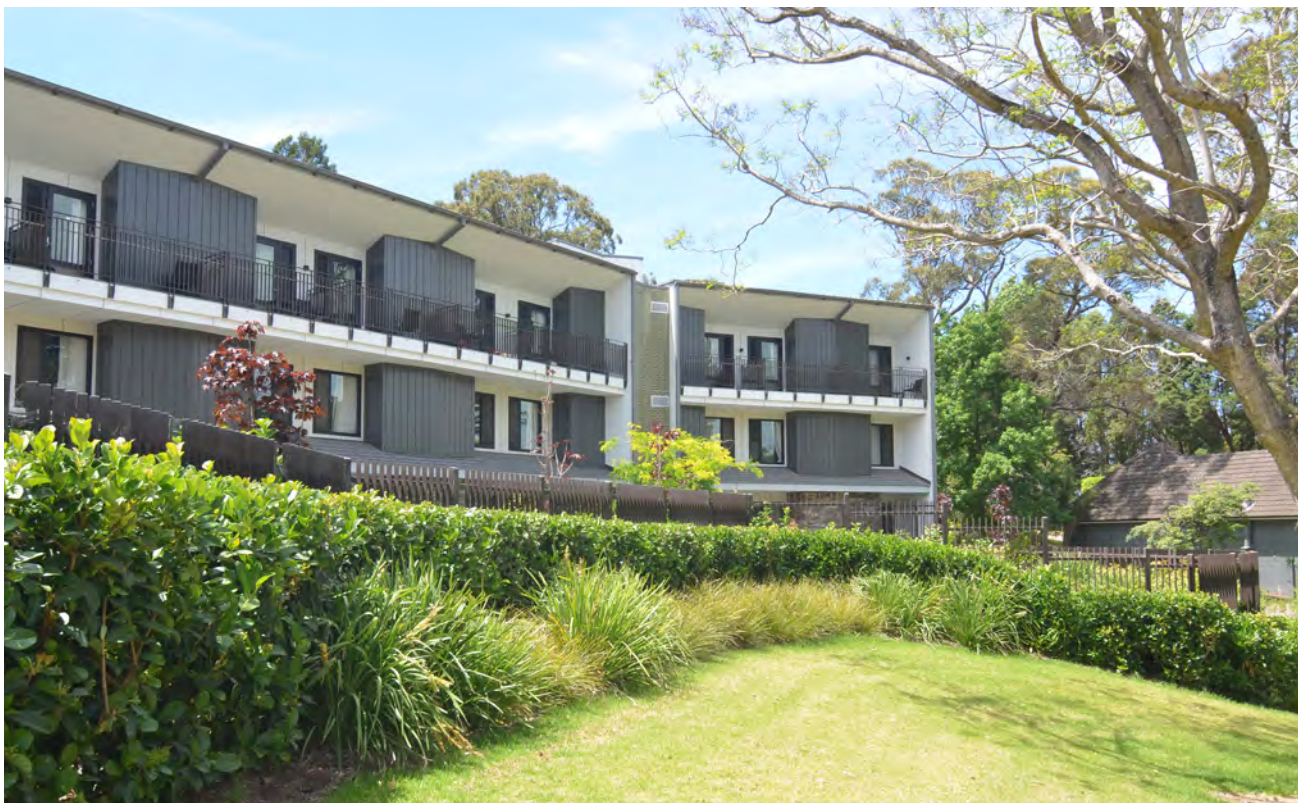
Fig 12.7.A Building and windows are angled away from neighbour's house and separated by generous landscaped setback and landscaping provides screening to courtyard spaces
