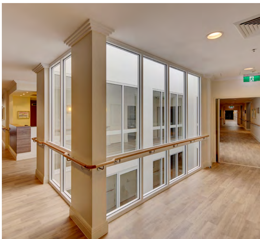
Fig 12.8.A Lightwells bring daylight and variance in light quality through the day into deep parts of the building in this residential care facility
