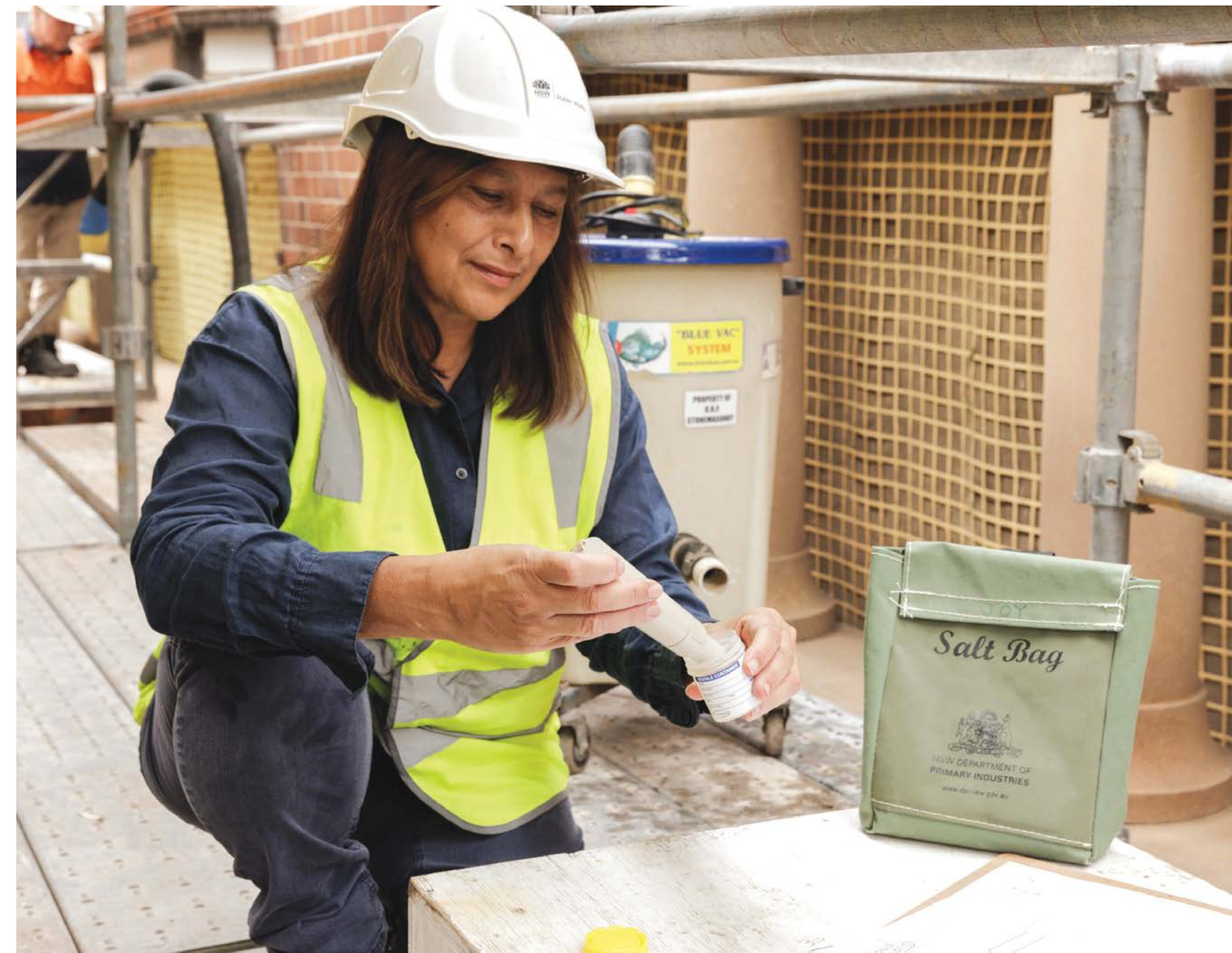
Below: Salt-level testing of captured water during stone desalination at Fort Street High School. Photograph by Sebastian Mrugalski, 2023
