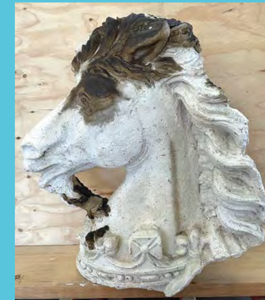
Plaster mould from a section of the Coat of Arms at the Local Central Court, Liverpool Street, Sydney. Photograph by Heritage Stoneworks 2023.
