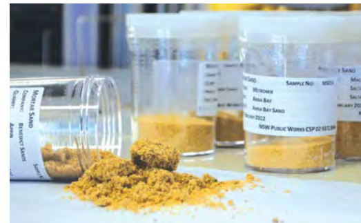
Below: Research into sourcing repointing sands was carried out in 2011 - 2013 and resulted in establishing a sand library to assist in specifying repointing mixes. Photograph by NSW Public Works, 2012.
